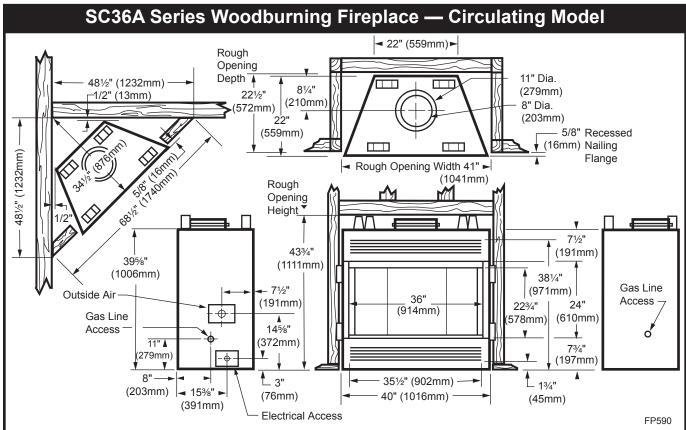
Fig. 2 SC36A Series specifications and framing.
